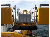
**Mobilisation:** The B2W system can be mobilized as a modular unit on the deck of any suitable vessel or be mounted on a deck pedestal for a permanent setup. The system is controlled from the deck or from an integrated control unit on the vessels bridge. Being hydraulically driven, the power can come from the vessel or from a separate hydraulic pack.
