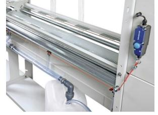
Steel bar with guiding spacers; comb (Recommended for easy cleaning)
