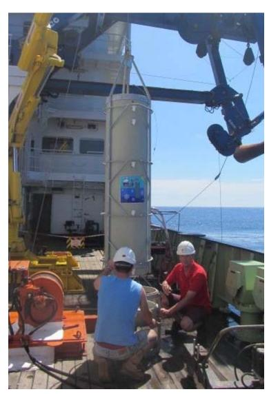
The Giant Marine Snow Catcher is a large volume water bottle that can be deployed to collect Marine Snow particles with the minimum of trauma.
