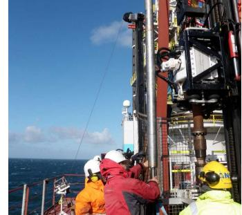
Due to the modular nature of the Orca it is a quick process to switch between CPT and sampling as well as changing from wireline to umbilical operation.
