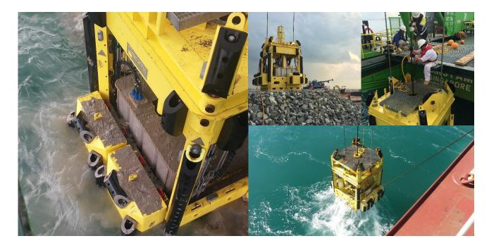
The Manta-200 represents Geomil Equipment's Cone Penetration Testing (CPT) system for seabed operations. Since its introduction in 2013 it has successfully completed challenging projects around the world and its performance is unsurpassed.
