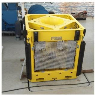
The Geomil Equipment Marlin-120 is a seabed template for support. Importantly the Marlin-120 has the ability to:
