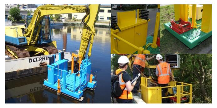
The Geomil Equipment Lizard-200 is a hitch-up Cone Penetration Testing (CPT) system to be used in combination with an excavator. It allows for conducting CPT's in near to impossible conditions, such as sites where space is limited and ground anchors cannot be used.
