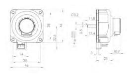
% There is a mounting screw hole with a depth of 3.5 mm with 3-M3 PCD  $\Phi28$  on the motor base side
