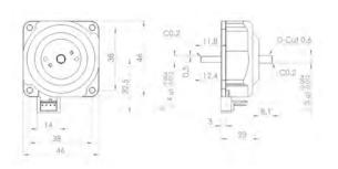
% There is a mounting screw hole with a depth of 3.5 mm with 3-M3 PCD  $\Phi28$  on the motor base side
