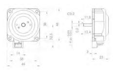
% There is a mounting screw hole with a depth of 3.5 mm with 3-M3 PCD  $\Phi 28$  on the motor base side
