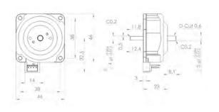
% There is a mounting screw hole with a depth of 3.5 mm with 3-M3 PCD  $\Phi28$  on the motor base side
