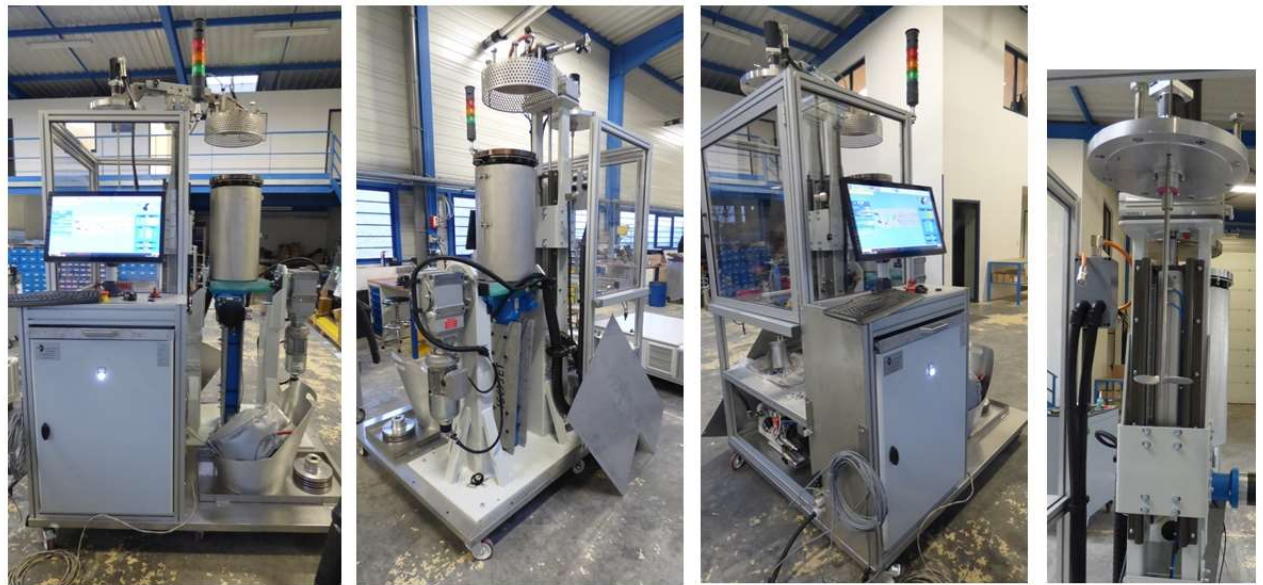
HT RTM Piston – T°C 300°C (310°C for regulation of heating elements) Included 1 heated cap for the 310°C mode
