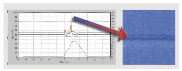
The most important quality parameter in texturing is the correct yarn tension. Abnormal tension levels and peaks result in dyeing problems.
