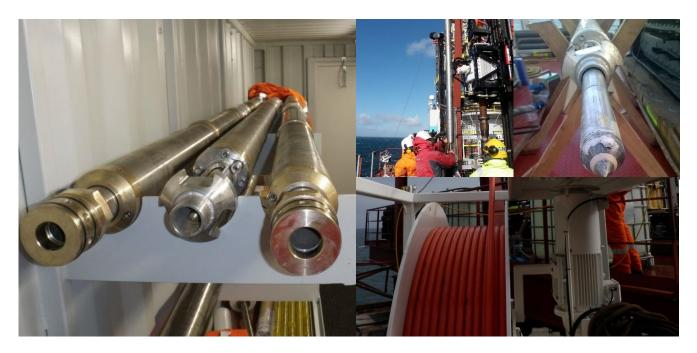
The Geomil Equipment Orca-125 is a versatile and fully integrated Cone Penetration Testing (CPT) testing and sampling system for downhole use. It is designed to be combined with several existing drilling methods.
