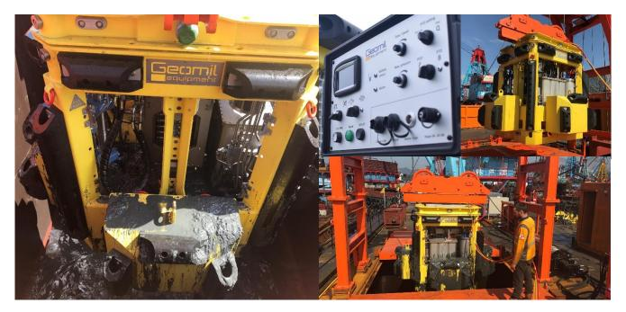
Geotechnical surveys are moving towards very deep waters. To provide operators with the best possible Cone Penetration Testing (CPT) equipment for these unique challenges, Geomil Equipment have developed the Manta-100 series.
