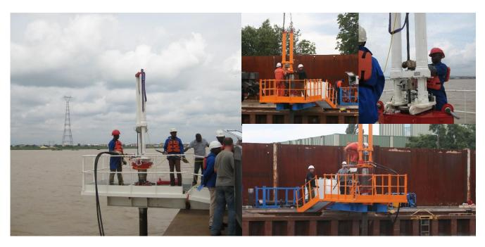
Geomil Equipment's Shark-200 is developed for nearshore and inshore Cone Penetration Testing (CPT) projects. Water depths from 2 to 30 m can be covered with great efficiency. The Shark-200 is ideal for CPT works in ports, waterways and channels.
